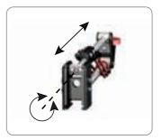
8) Position the swivel adjustment of the arm fitting. At the bottom of the arm fitting - between the two screws - a sunken bolt is located (a). This bolt fixates the sliding plate, that is connected to the arm fitting, to the double joint. By moving the
