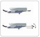
11) The horizontal movements of the extension arms can be limited if desired. This is done by putting a synthetic plug into the bottom of the extension arm. Blocking pins are then put in the pattern of holes of the underlying extension arm (or in the top of the rotation block), according to the area that has to be limited. Now, the extension arms can only rotate within the area that is limited by the pins. By limiting the rotation area of the extension arms, some improved
